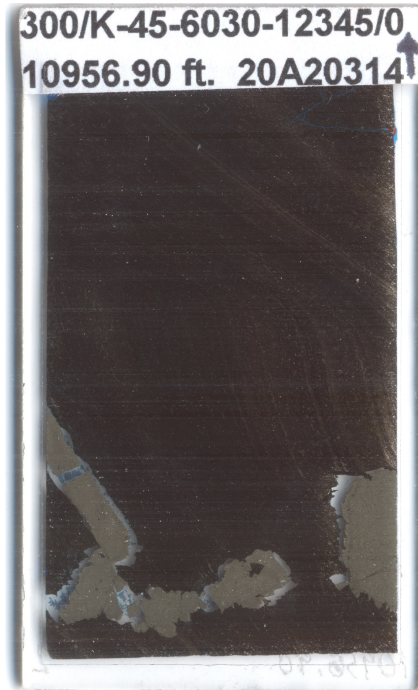
Figure 11A: Thin section scan of sample T38 collected from the Nahanni Formation at the 300/K-45-6030-12345/0 location. The sample is classified as silicified dolomitic shale with vertical to subvertical dipping and folded laminations. The lower portion show large vertical to horizontal fractures and voids occluded with pyrite, chalcedony and ferroan carbonate (calcite and dolomite).
